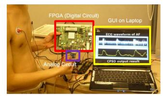
**Figure 6** The ECG signals are amplified and filtered by the in-house instrument amplifier IC. Then the A/D converter on FPGA board converts the analog ECG into digital samples at 256 samples per second (sps). Afterwards, the proposed digital system with ASP and GPP performs the CPSD calculation. The FPGA is connected to a laptop with RS-232, and the filtered raw data as well as the CPSD index are fetched and displayed with GUI on the screen.
