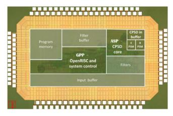
Figure 7 90 nm digital part chip photo.
